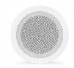
Ceiling loudspeaker for PA. Features: Provides crystal-clear sound, perfect for voice and background music. Manufactured in ABS with a steel grille that ensures its durability. It is quick and easy to install, minimizing assembly time. Applications: Background music and voice announcements in 100V line installations for offices, shops, restaurants, waiting rooms, etc. Technical data: 5" double cone loudspeaker 6/3 W RMS@100 V Response 140-15,000 Hz Sensitivity 90 dB at 1 W/1 m
