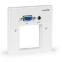
Integrated connection panel with VGA connectors and 3.5 mm stereo jack with window for 1 connection panel. Connection using screw terminal blocks. Compatible with the WP modular connection panel system.
