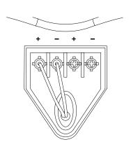
Connect the positive (+) and negative (-) speaker cable to the left + and right - screw terminals.
