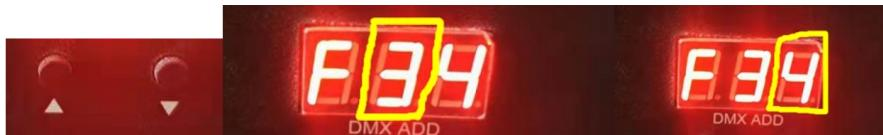
The first number on the display indicates the number of the machine, in the example the 3 indicates that this is the third machine.
